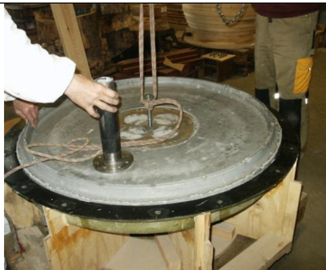
The top is taking out of the mould
