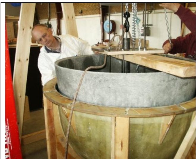
Taking the float out of the mould
