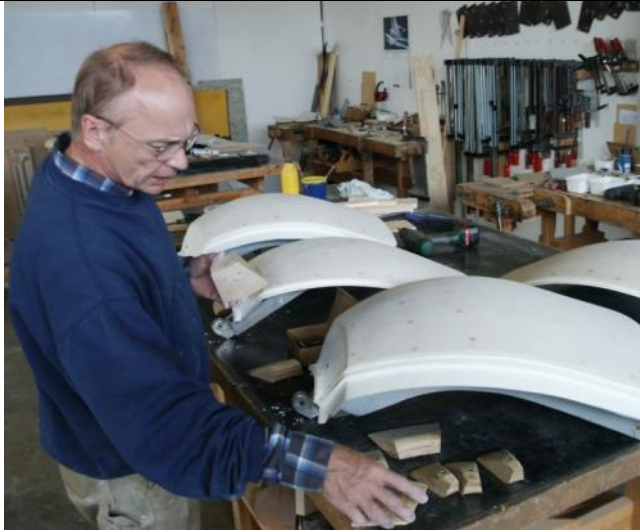
Preparation of the internal mould
