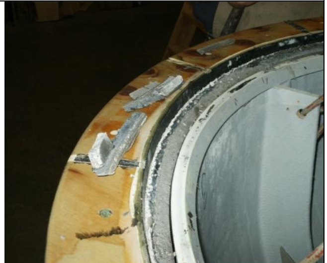
Critical operation to separate the mould
