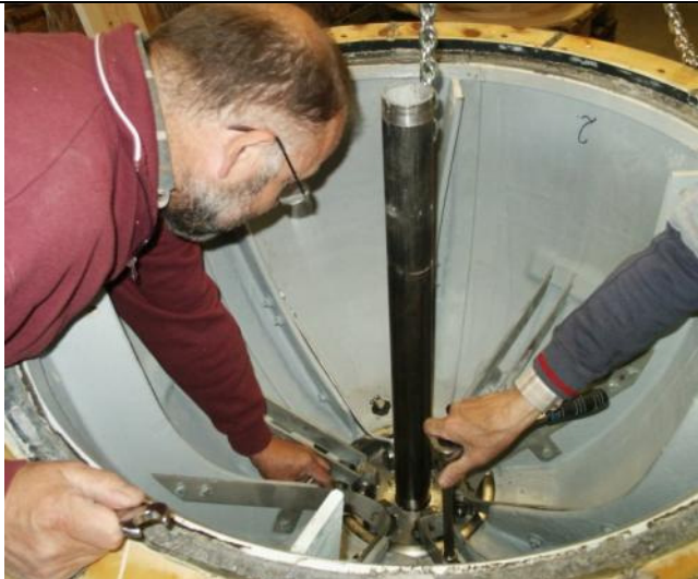
Dismounting of the outside mould
